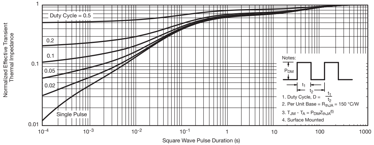
Normalized Thermal Transient Impedance, Junction-to-Ambient
