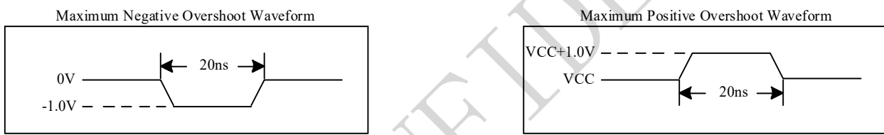
Figure 5-1 Maximum Overshoot Waveform
