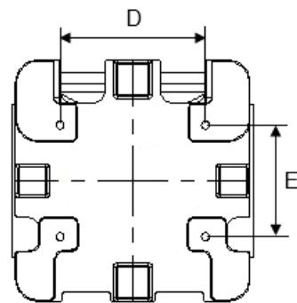
PCB aperture  $\geq \Phi 1.4\text{mm}$
