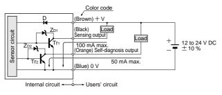
Symbols ... D: Reverse supply polarity protection diode Z<sub>D1</sub>, Z<sub>D2</sub>: Surge absorption zener diode Tr<sub>1</sub>, Tr<sub>2</sub>: NPN output transistor
