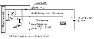
Symbols ... D: Reverse supply polarity protection diode Z<sub>D1</sub>, Z<sub>D2</sub>: Surge absorption zener diode Tr<sub>1</sub>, Tr<sub>2</sub>: PNP output transistor
