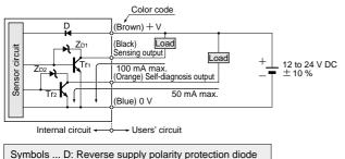
Symbols ... D: Reverse supply polarity protection diode Z<sub>D1</sub>, Z<sub>D2</sub>: Surge absorption zener diode Tr<sub>1</sub>, Tr<sub>2</sub>: NPN output transistor
