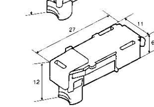
\*The material is PBT for housing and color of plug housing is yellow. \*The figures in □ vary according to housing color.
