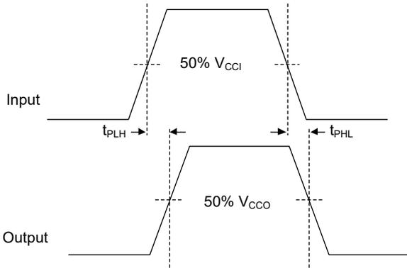
Figure 3. Propagation Delay
