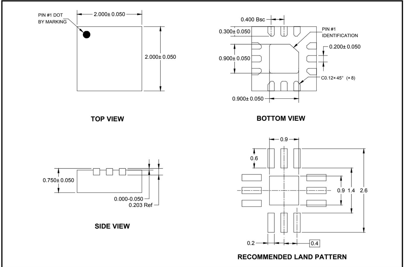
NOTE: All linear dimensions are in millimeters.
