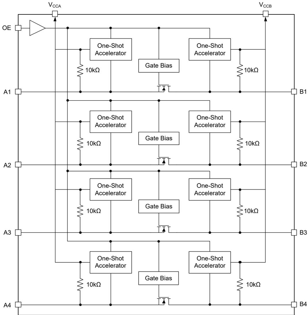
Figure 2. Block Diagram
