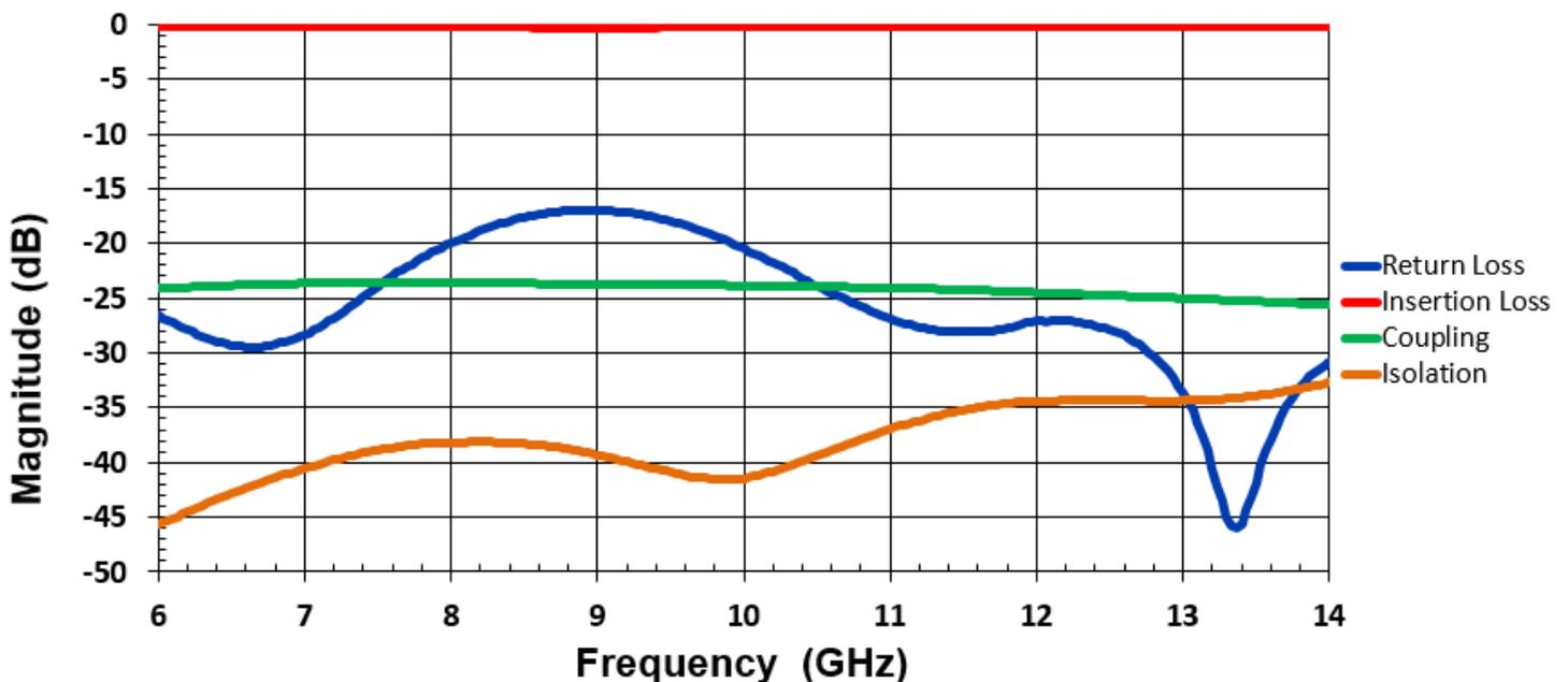
\*Typical measured performance mounted on RO4350B test board at 25°C.
