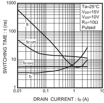
Fig.2 Switching Characteristics
