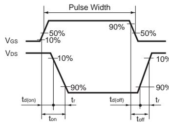
Fig.1-2 Switching Waveforms
