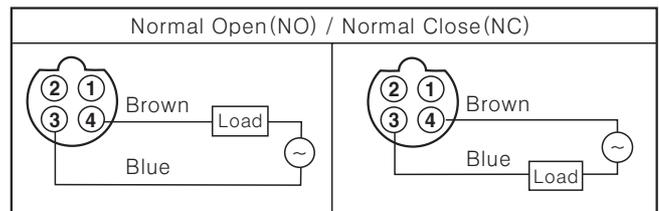
\*In AC inductive type, ② and ③, ① and ④ are connected inside of the connector cable.
