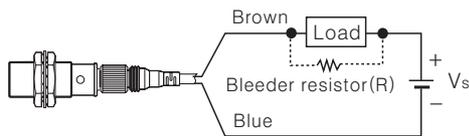
Please make the current on proximity sensor smaller than the return current of load by connecting a bleeder resistor in parallel.
