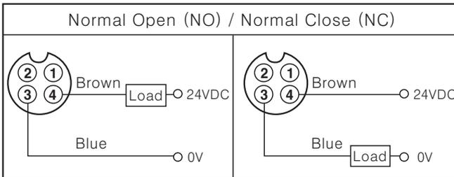
\*Pin ①, ② are N.C (Not Connected) terminals.
