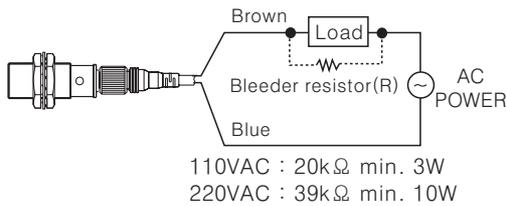
It may cause return failure of load by residual voltage. If the load current is under 5mA, please make sure the residual voltage is less than the return voltage of the load by connecting a bleeder resistor in parallel with the load as shown in the diagram.
