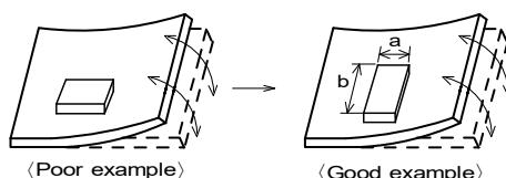
(2) Components location on PCB separation
