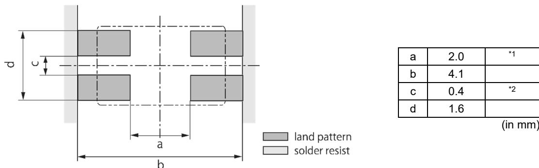
\*1 If the pattern is made wider than the specified dimensions, the strength of bending will be reduced. Also, if the pattern is made smaller than the specified dimensions, a short circuit may occur.
