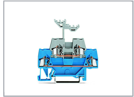
Double-deck terminal blocks accommodate two circuits of different potentials on two decks; different circuits can be differentiated by color coding either deck (280 Series). The lower deck is wider than the upper for easier wiring.
