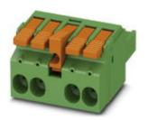
PCB connector, nominal current: 41 A, number of positions: 6, pitch: 7.62 mm, connection method: Push-in spring connection, color: green, contact surface: Tin
