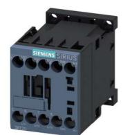
power contactor, AC-3e/AC-3, 9 A, 4 kW / 400 V, 3-pole, 24 V DC, auxiliary contacts: 1 NC, screw terminal, size: S00
