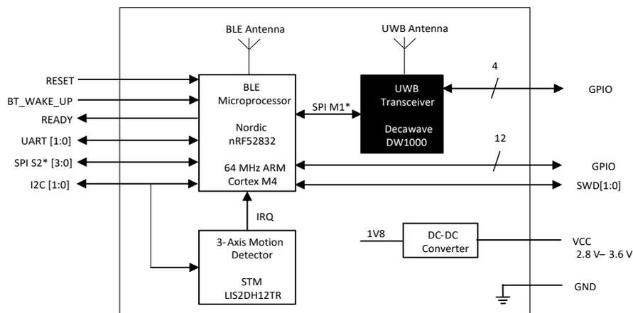
\*SPI M1 is nRF52 SPI master 1, SPI S2 is SPI slave 2
