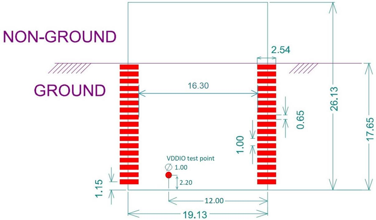
Figure 6: DWM1001 Module Land Pattern (units: mm)
