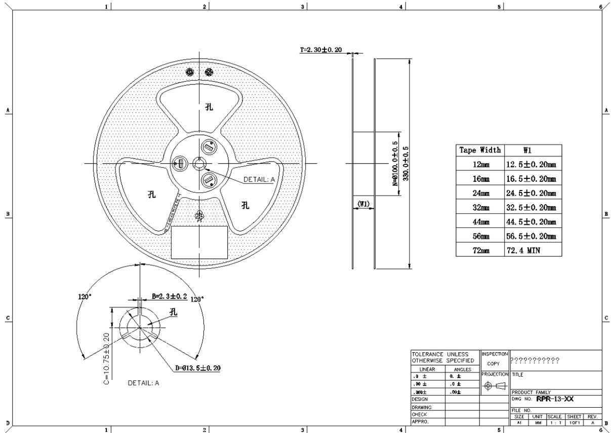
Figure 8: DWM1001 Tape and Reel Dimensions
