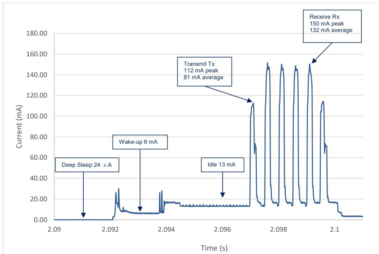
**Figure 2: Power consumption running PANS R2 tag application
