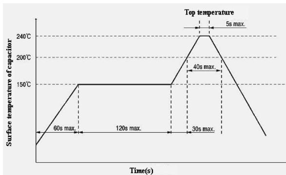
Recommended curve for lead free soldering is as following.
