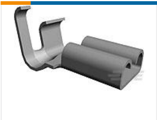
TE Part #1217244-2 187 FASTON,FLAG,REC.,18-14 AWG, TPBR
