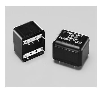
This Coilcraft current sense transformer is intended for use in measuring 50/60 Hz line currents from 0.5 to 20 Amperes rms. Typical application shown below yields an output of 0.1 Volt per Ampere. The sensitivity may be changed by adjusting the value of the terminating resistance (R<sub>T</sub>). These parts also can be used to measure 400 Hz line currents.
