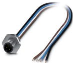
Flush-type connector, Universal, 4-position, PlugLink:M12, A-coded, Front mounting, M16 x 1.5, Individual wires, Cable length: 0.5 m
