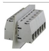
Panel feed-through terminal block, connection method: Screw connection, number of positions: 1, load current: 150 A, cross section: 16 mm² - 50 mm², AWG 6 - 1/0, connection direction of the conductor to plug-in direction: 0 °, width: 18.8 mm, color: gray
