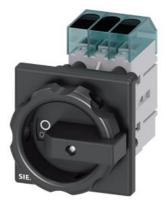
Load disconnector 3LD3, lu 25 A Main switch 3-pole Rated operating capacity at AC-23 A at 400V 9.0kW Front plate mounting Basic switch with Central hole mounting 22.5mm Toggle drive black 66x66 mm
