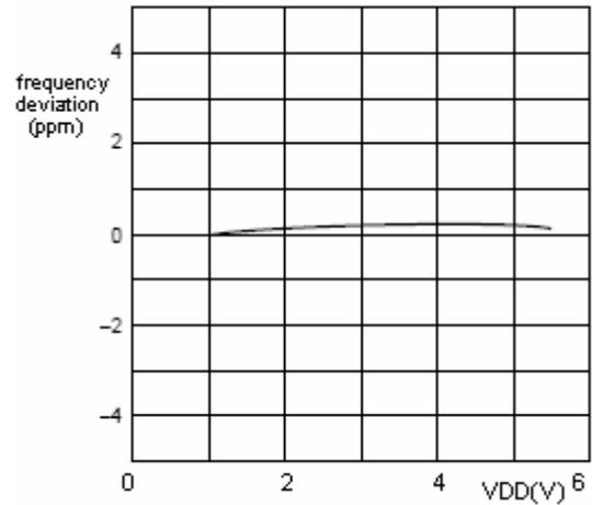
T<sub>amb</sub> = 25°C; normalized to VDD = 3V.
