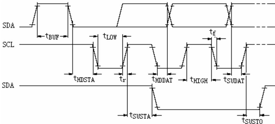
**Figure1: I<sup>2</sup>C-bus timing waveform**
