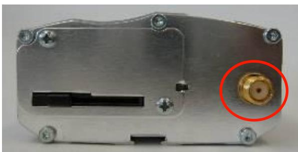
Figure 23. Main RF Connector for the FXT001, FXT002, FXT009 and FXT010
