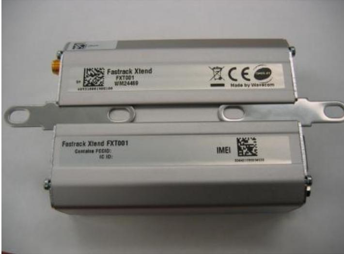
Figure 43. Fastrack Xtend Holding Bridles
