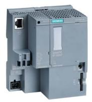
SIMATIC DP, CPU 1510SP-1 PN for ET 200SP, Central processing unit with Work memory 100 KB for program and 750 KB for data, 1st interface: PROFINET IRT with 3-port switch, 72 ns bit performance, SIMATIC Memory Card required, BusAdapter required for Port 1 and 2
