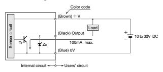
Symbols ... Zp: Surge absorption zener diode Tr : NPN output transistor
