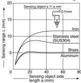
As the sensing object size becomes smaller than the standard size (iron sheet  $40\times40\times11$ mm), the sensing range shortens as shown in the left figure.
