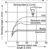
As the sensing object size becomes smaller than the standard size (iron sheet  $25\times25\times$ t1mm), the sensing range shortens as shown in the left figure.
