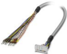
Round cable set; connection 1: Single wires (14-position) (The wires are marked and fitted with ferrules.); connection 2: IDC/FLK socket strip (1x 14-position); cable length: 1 m
