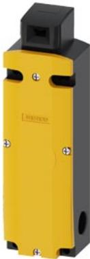
Safety position switch with tumbler Locking force 1300 N 5 directions of approaches Solenoid-locked Magnet voltage 24 V DC Monitoring actuator 2 NC/1 NO Monitoring magnet 2 NC/1 NO The matching separate actuator 3SE5000-0AV0. must be ordered separately
