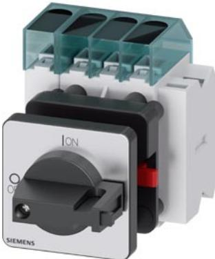
Load disconnector 3LD3, Iu 25 A Main switch 3-pole + N Rated operating capacity at AC-23 A at 400V 9.0kW Front plate mounting Basic switch with Central hole mounting 22.5mm Toggle drive black 48x48 mm with auxiliary switch 1OE + 1S
