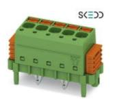
PCB direct plug, nominal current: 12 A, rated voltage (III/2): 320 V, number of positions: 5, pitch: 5 mm, connection method: Push-in spring connection, color: green, contact surface: Tin, mounting: SKEDD - Direct plug-in technology
