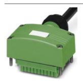
Connector hood, application: Sensor/actuator box, connection method: M12-SPEEDCON-socket Metal, number of slots: 4, slot assignment: Double, status display: No; master cable connection: Pluggable screw connection 180°, PUR/PVC, cable length: 10 m, shielding: no
