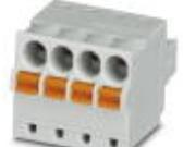
PCB connector, nominal current: 8 A, rated voltage (III/2): 160 V, Nominal cross section: 1.5 mm<sup>2</sup>, number of positions: 5, pitch: 3.5 mm, connection method: Push-in spring connection, color: light gray, contact surface: Tin
