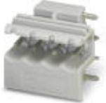
PCB headers, number of positions: 4, pitch: 5 mm, color: light gray, contact surface: Tin, Pin layout: Linear pinning, solder pin [P]: 3.5 mm, Article with lateral pin exit
