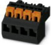
PCB connector, number of positions: 4, pitch: 5 mm, color: black, contact surface: Tin
