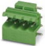
PCB headers, number of positions: 4, pitch: 5 mm, color: green, contact surface: Tin, Pin layout: Linear pinning, solder pin [P]: 3.5 mm, Article with lateral pin exit
