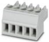
PCB connector, nominal current: 8 A, rated voltage (II/II): 160 V, Nominal cross section: 1.5 mm<sup>2</sup>, number of positions: 5, pitch: 3.5 mm, connection method: Screw connection with tension sleeve, color: light gray, contact surface: Tin
