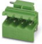
PCB headers, number of positions: 4, pitch: 5 mm, color: green, contact surface: Tin, Pin layout: Linear pinning, solder pin [P]: 3.5 mm, Article with lateral pin exit
