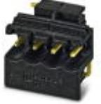
PCB headers, number of positions: 4, pitch: 5 mm, color: black, contact surface: Gold, Pin layout: Linear pinning, solder pin [P]: 2.5 mm, Article with lateral pin exit
