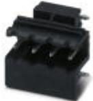
PCB headers, number of positions: 4, pitch: 5 mm, color: black, contact surface: Tin, Pin layout: Linear pinning, solder pin [P]: 3.5 mm, Article with lateral pin exit
