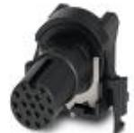
Sensor/actuator flush-type socket, 17-pos. with shroud, A-coded, with angled solder connection, contact insert only
