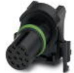
Sensor/actuator flush-type socket, 12-pos. without shroud, A-coded, with angled solder connection, contact insert only
