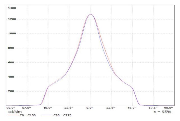
Luminaire: LEDiL Oy C13660\_ANGELINA-M-B\_(BXRA\_ES) Eff. 92% Lamps: 1 x Bridgelux BXRA\_ES\_(QQ40\_BXRA-W1202\_1019A-2010) 268Im@250mA\_P=3.36W\_I=250mA
