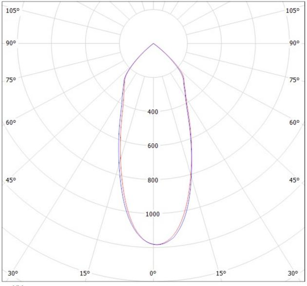
cd/klm \_\_\_\_\_\_ C0 - C180 \_\_\_\_\_ C90 - C270
