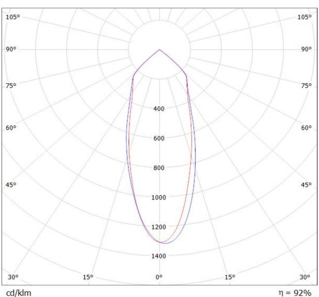
Luminaire: LEDiL Oy C13660\_ANGELINA-M-B\_(BXRA\_ES) Eff. 92% Lamps: 1 x Bridgelux BXRA\_ES\_(QQ40\_BXRA-W1202\_1019A-2010) 268Im@250mA\_P=3.36W\_I=250mA
