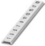
Zack Marker strip, flat, Strip, white, labeled, printed horizontally: Odd numbers 1 - 19, 21 - 39, etc. up to 81 - 99, mounting type: snap into flat marker groove, for terminal block width: 5 mm, lettering field size: 5.15 x 5.15 mm
