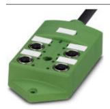
Sensor/actuator box, application: Standard, connection method: M12-SPEEDCON-socket Metal, number of slots: 4, number of positions: 4, coding: A - standard, slot assignment: single, status display: yes, pnp; master cable connection: Fixed connection 180°, PUR/PVC, cable length: 10 m, shielding: no
