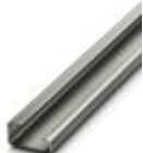
DIN rail, unperforated, G profile, width: 32 mm, height: 15 mm, acc. to EN 60715, material: Steel, galvanized, passivated with a thick layer, length: 2000 mm, color: silver
