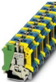
Installation ground terminal block, Screw connection, cross section: 2.5 mm<sup>2</sup> - 25 mm<sup>2</sup>, AWG: 12 - 4, width: 24 mm, color: green-yellow-blue, mounting type: NS 35/7,5, NS 35/15, NS 32
