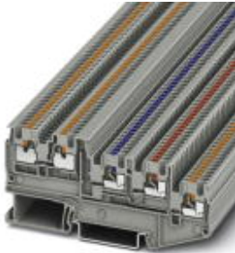
Sensor/actuator terminal block, with green light indicator, Connection method: Push-in connection, Cross section: 0.14 mm 2 - 1.5 mm 2 , AWG: 26 - 14, Width: 3.5 mm, Color: gray, Mounting type: NS 35/7,5, NS 35/15
