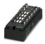
The local bus device has digital inputs. Functions: 16 digital inputs, 3 ms filter time, 500 kbaud/2 Mbaud selection, channel-specific diagnostics, short-circuit and overload protection, 1.2 A nominal current, M12 fast connection technology.
