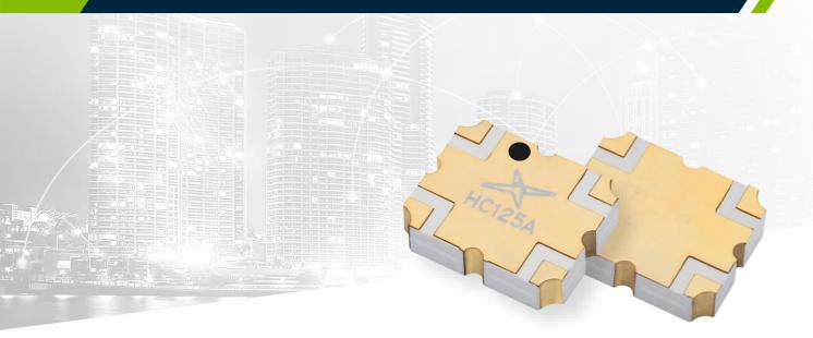
The Taoglas HC125A is a low profile, high performance, 3dB hybrid coupler in an easy to integrate surface mount package. It is designed for multi feed GNSS applications. The HC125A is particularly used for applications where balanced power and low noise amplifiers are required. It has low insertion loss and tight amplitude and can be used in power applications up to 30 Watts. It has been engineered to cover the full GNSS bandwidth of 1150 – 1630MHz.
