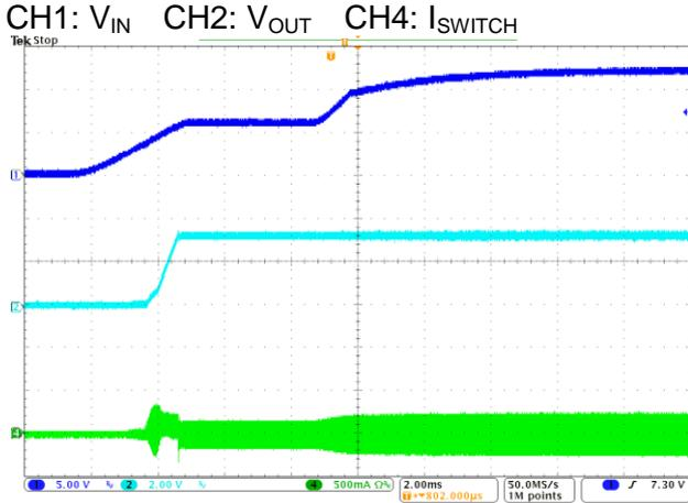
$V_{IN}$  Power On Waveform ( $I_{LOAD}=0A$ )
