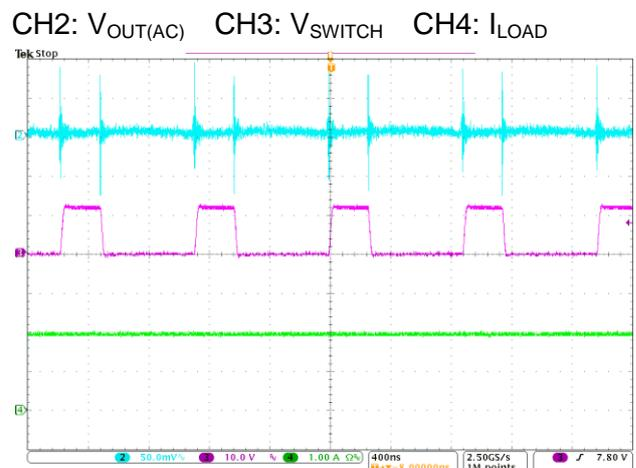
Heavy Load Output Ripple Waveform
