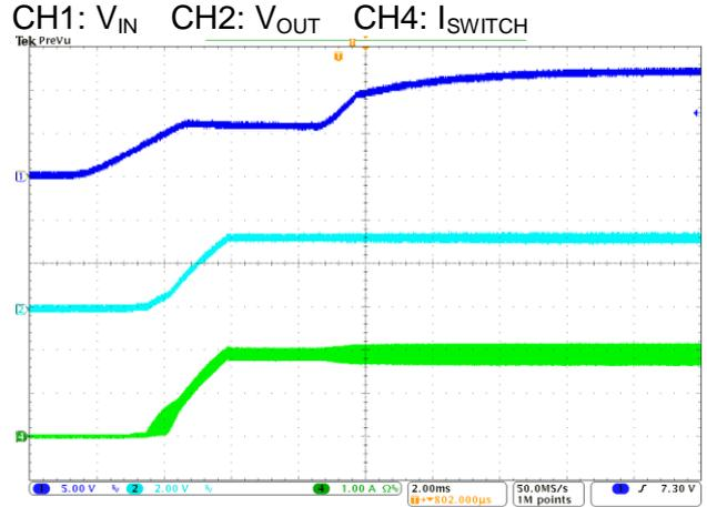
$V_{IN}$  Power On Waveform ( $I_{LOAD}=2A$ )
