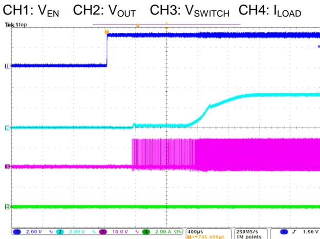
$V_{EN}$  Power On Waveform ( $I_{LOAD}=0A$ )
