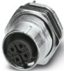
Sensor/actuator flush-type socket, 5-pos., M12-SPEEDCON, A-coded, rear/screw mounting with Pg9 thread, with straight solder connection, design with 12 mm long solder pins
