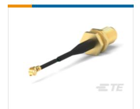
TE Model / Part # 2032440-1 C/A, UMCC TO SMA BHD JACK, 1.37 MM L200MM
