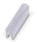
Conductor marker carrier, transparent, unlabeled, Mounting type: slide on, Cable diameter: 1.5-2.5 mm, Lettering field:  $4 \times 15$  mm
