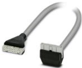
Round cable set; connection 1: IDC/FLK socket strip (1x 20-position, 180 °-Out put); connection 2: IDC/FLK socket strip (1x 20-position, 90 °-out put); cable length: 1 m
