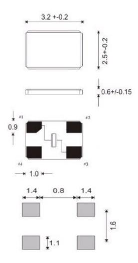
Note: Due to material availability, the chamfer could be located on pin #1, 3, or 4. Be advised that the chamfer location has no impact on the electrical performance of the device.
