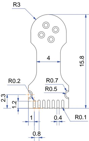
Figure 4. Flex outline. All dimensions are in [mm].
