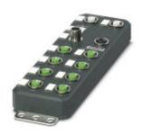
Axioline E, Digital I/O device, PROFINET, M12 fast connection technology, Digital inputs: 8, 24 V DC, connection method: 4-wire, Digital outputs: 4, 24 V DC, 2 A, connection method: 3-wire, Plastic housing, degree of protection: IP65/67
