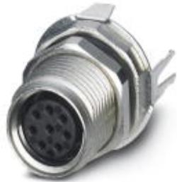
Sensor/actuator flush-type connector, socket, 8-pos. M8, rear/screw mounting with M10 fastening thread, with straight solder connection
