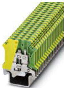
Ground modular terminal block, Connection method: Screw connection, Number of positions: 1, Cross section: 0.2 mm<sup>2</sup> - 4 mm<sup>2</sup>, AWG: 24 - 12, Width: 6.2 mm, Color: green-yellow, Mounting type: NS 35/15-2,3
