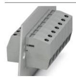
Panel feed-through terminal block, Connection method: Screw connection, Load current: 125 A, Cross section: 6 mm² - 35 mm², AWG 10 - 2, Connection direction of the conductor to plug-in direction: 0 °, Width: 15.1 mm, Color: gray
