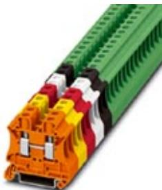
Feed-through terminal block, Connection method: Screw connection, Cross section: 0.2 mm<sup>2</sup> - 10 mm<sup>2</sup>, AWG: 24 - 8, Width: 8.2 mm, Color: black, Mounting type: NS 35/7,5, NS 35/15
